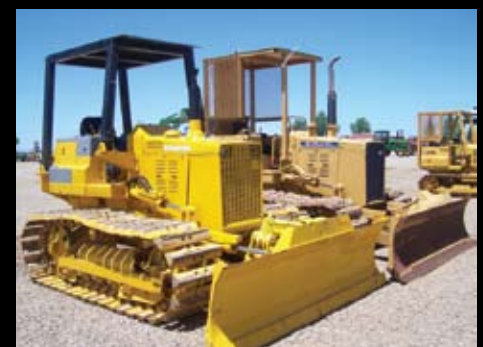
2 KOMATSU D 31 P DOZERS w/6 WAY BLADES
